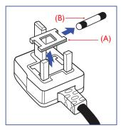
This apparatus is supplied with an approved moulded 13A plug. To change a fuse in this type of plug proceed as follows:
