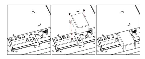
Maximum USB stick size recommended: 43BDL3017P / 50BDL3017P: 20(W)x10(H)x60(L) mm 55BDL3017P: 20(W)x10(H)x45(L) mm
