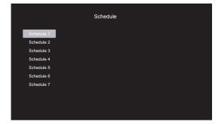
Press [<sup>∩</sup>] or [<sup>¬</sup>] button to select a schedule item (item number 1 - 7), and press [OK] or [<sup>¬</sup>] button to enter the submenu.
