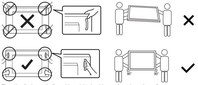
· Place the display vertically and its weight should spread evenly on the surface.
