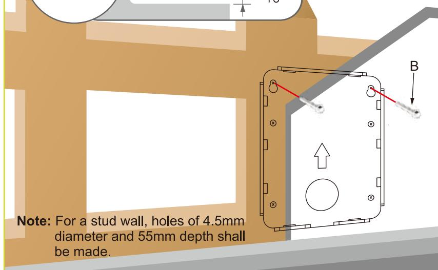
**Note:** For a stud wall, holes of 4.5mm diameter and 55mm depth shall be made.
