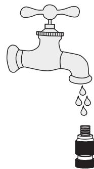
for gel spray, When it is blocked, you can take the nozzle down and wipe it with water.
